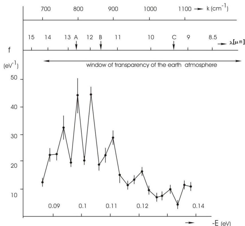
*Figure 5.* NES-spectrum of deionized water (chemical purity – 99,99 %; pH – 6,5–7,5; total mineralization – 200 mg/l; electric conductivity – 10  $\mu\text{S}/\text{cm}$ ). The horizontal axis shows the energy of the H...O hydrogen bonds in the associates –  $E$  (eV). The vertical axis – energy distribution function –  $f$  ( $eV^{-1}$ ).  $k$  – the vibration frequency of the H–O–H atoms ( $\text{cm}^{-1}$ );  $\lambda$  – wavelength ( $\mu\text{m}$ )
