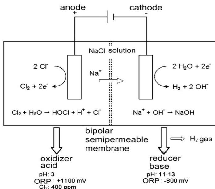
Figure 1. The diaphragm electrolysis method for the preparation of acid (anolyte) and alkali (catholyte) solutions via the electrochemical activation of sodium chloride
